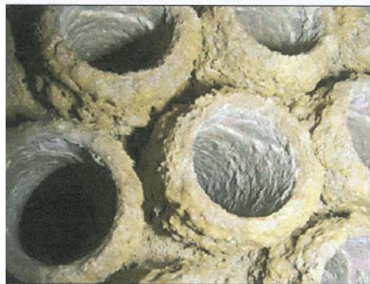
Figure 1. Improper application of biocides can result in biofouling.
