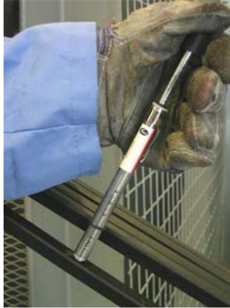
Figure 3. The tension gauge should be used for proper drive tensioning.
