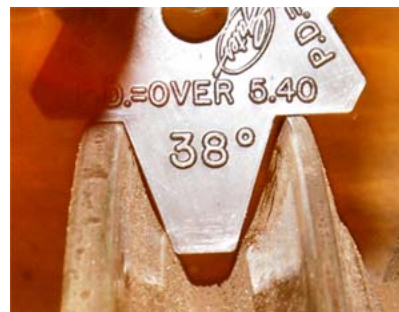
Figure 2. Use a groove gauge to help visualize sheave wear.
